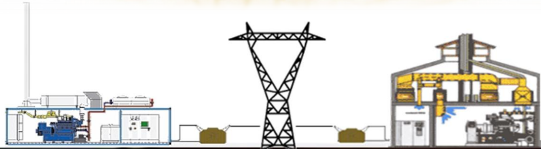
Natural Gas Cogeneration Power Module or alternatively Inside Gas Cogeneration Installation
